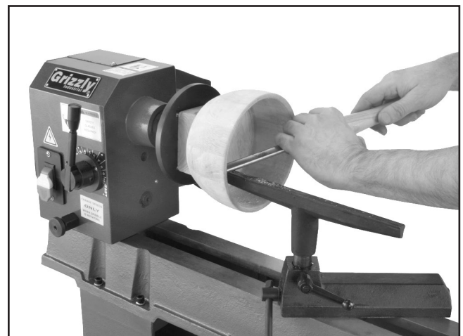
Figure 27. Typical faceplate turning operation.
